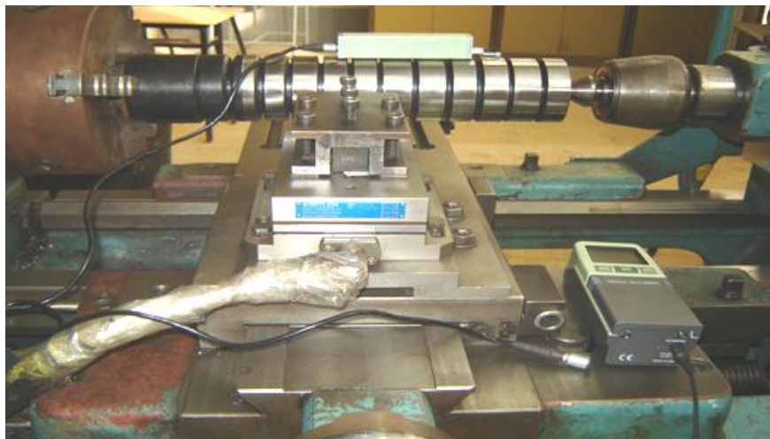
Fig. 1 (a) Surftest 201 Mitutoyo, (b) Expérimental configuration for measuring surface roughness
