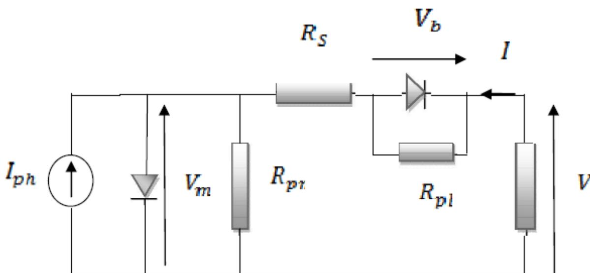
Figure 3: Equivalent electrical circuit of a cell exhibiting a S-shaped J-V curve.
