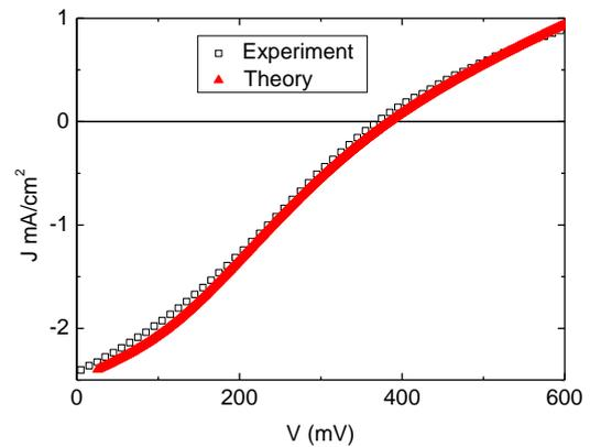
Figure 4: J–V characteristics under AM1.5 illumination of a solar cell using a MA(11 nm)/CuI anode structure (■) experimental and (▲) theoretical curves.
