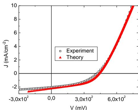
Figure 2: J–V characteristics under AM1.5 illumination of a solar cell using a MA(17 nm)M/Au/CuI anode structure (■) experimental and (▲) theoretical curves.
