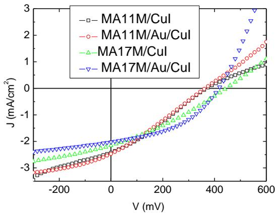
Figure 1: J-V characteristics of OPVCs with different anodes.
