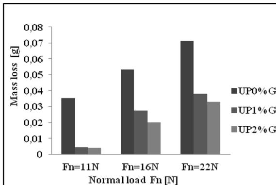
Fig.7 : Mass loss versus normal load for the three compositions at  $V_g = 0.32\text{m/s}$ .
