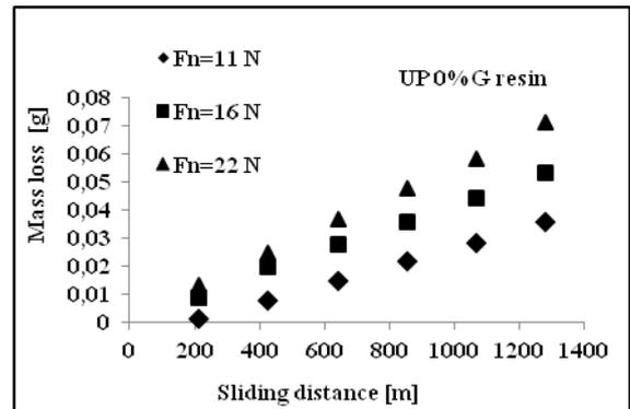
Fig. 6 : Mass loss as a function of the sliding distance for the UP0%G resin at  $V=0.32\text{m/s}$ .
