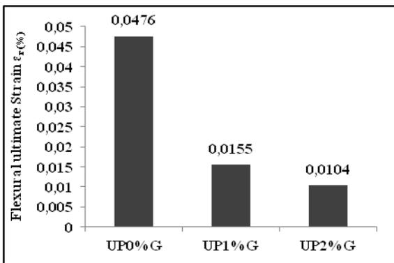
Fig. 3 : Strain at failure versus graphite percentage.
