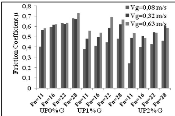
Fig. 5 : Coefficient of friction versus the Normal load  $F_n$  and the sliding speed  $V_g$  for the three studied compositions.
