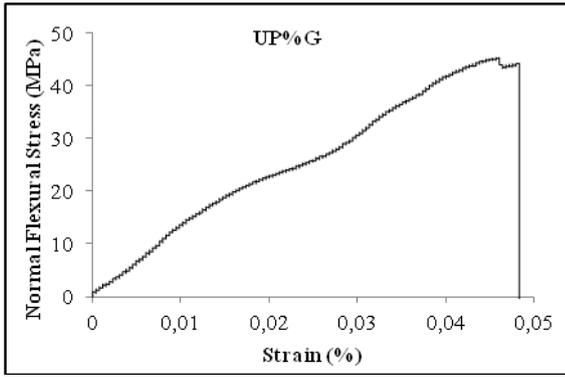
Fig. 1: Normal Flexural Stress versus Strain for UP0%G.
