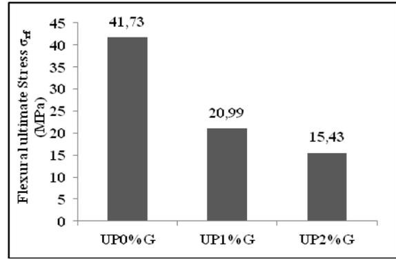
Fig. 2: Stress at failure versus the graphite percentage.
