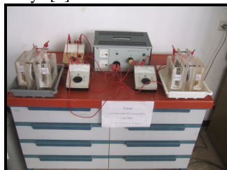
Fig 01: Model of the permeability test to the ions chlorinates[5]
