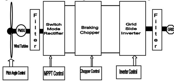
Figure 1.VSWT System Structure and Control
