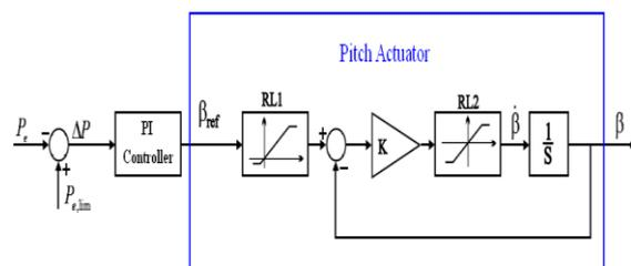
**Figure 6.** Pitch controller system model
