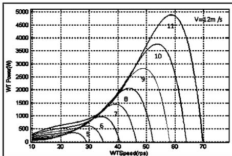
Figure 2.Wind Turbine Power versus speed [2]
