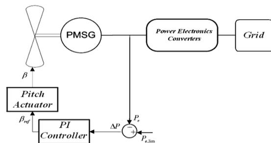
**Figure 5.** Block diagram of pitch control system
