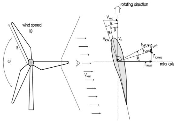
**Figure 4.** Aerodynamic forces at a rotor blade [8]
