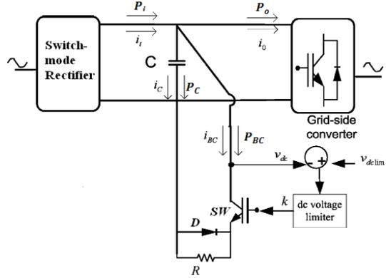
Figure 8. DC bus model highlighted [9]
