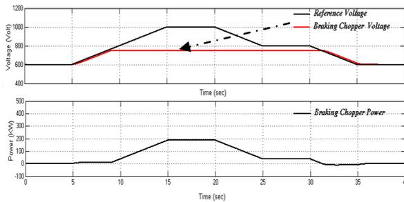
**Figure 10.**Braking Chopper voltage and power
