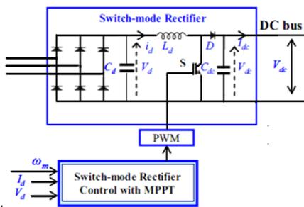
Figure 3.Switch-mode rectifier structure [3]
