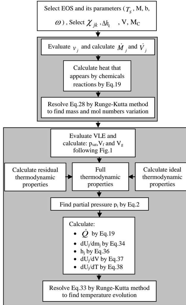
Fig. 1 Diagram of Thermal-Hydraulic Analysis
