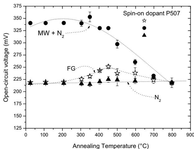
**Figure 4.** Open-circuit voltage vs annealing temperature under forming gas or pure nitrogen of hydrogenated and non-hydrogenated  $n^+pp^+$  poly-Si mesa structures. The annealing time is 30 min.
