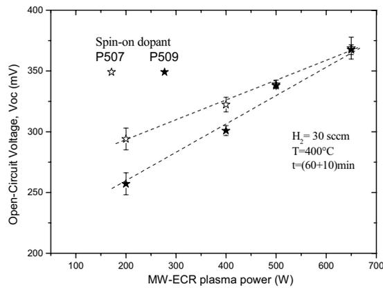
**Figure 1.** Influence of MW-ECR plasma power on open-circuit voltage measured on the  $n^+pp^+$  mesa cells. The hydrogenation conditions are indicated.
