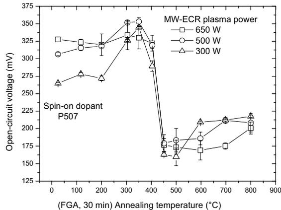
**Figure 3.** Open-circuit voltage versus forming gas annealing temperature of MW-ECR plasma hydrogenated  $n^+pp^+$  poly-Si mesa structures. The FG annealing time is 30 min.
