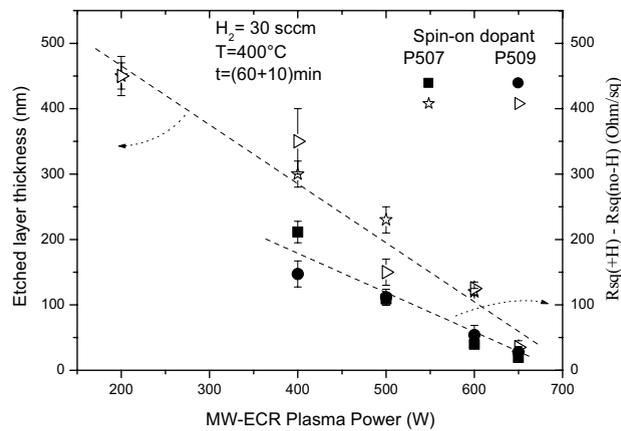
**Figure 2.** Etched layer thickness and the difference in emitter sheet resistance without and with hydrogenation versus MW-ECR plasma power as a function of the plasma power
