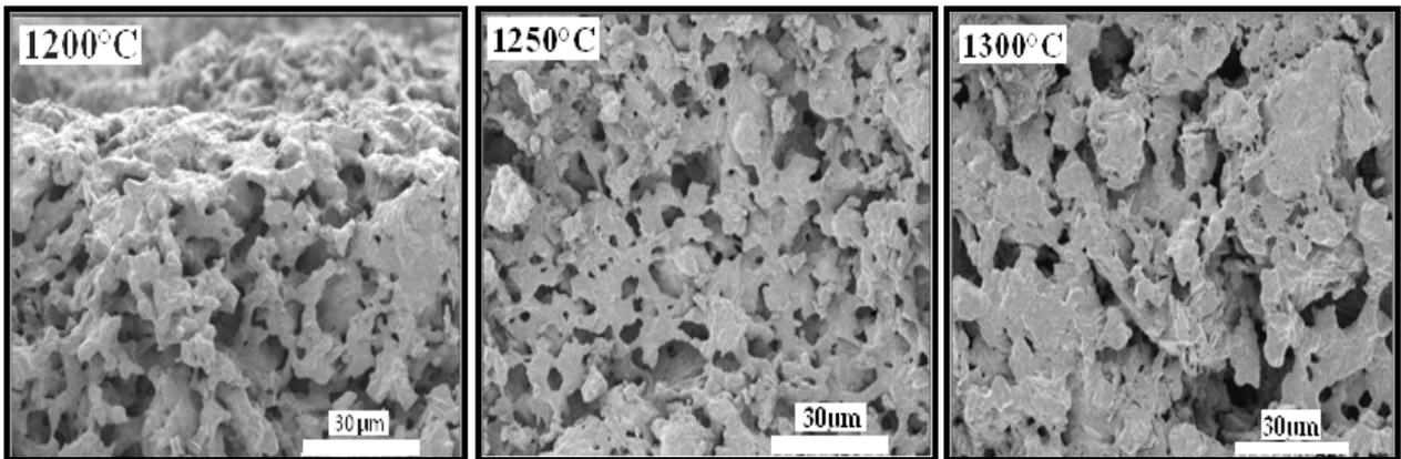
Fig. 3. SEM micrograph of the cross-section of supports in samples sintered at 1200°C, 1250°C and 1300°C for 1h.
