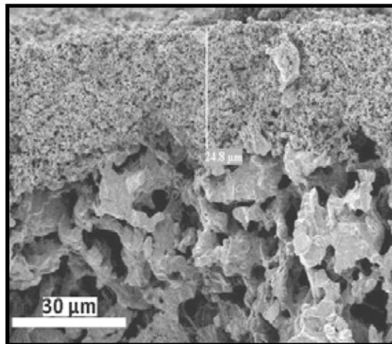
Fig. 6. SEM micrograph of the cross-section of both membrane and support
