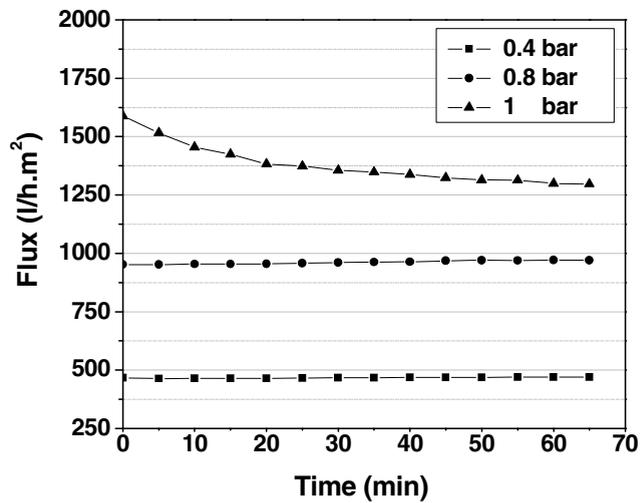
Fig. 7. Water flux as a function of time for 3 working pressure values.
