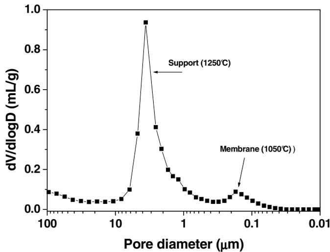
Fig. 5. Pore size distribution of support + membrane.
