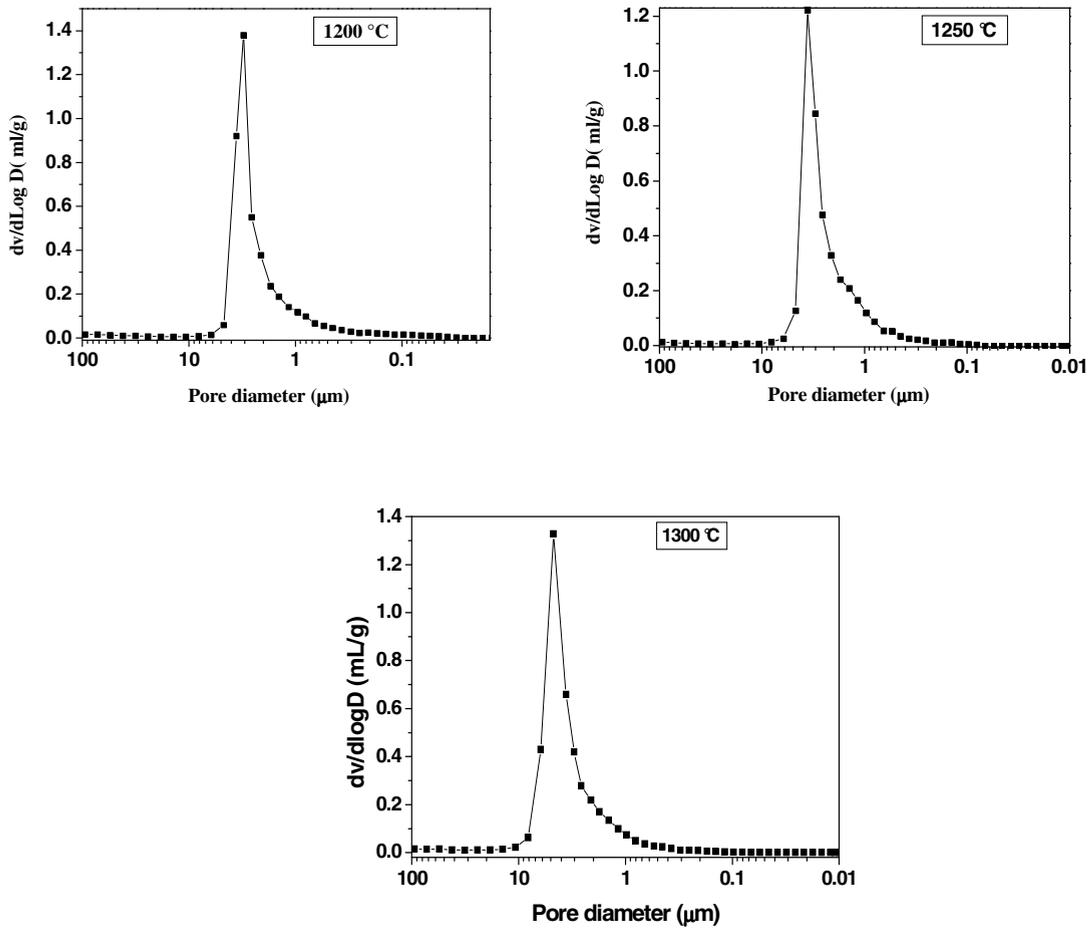
Fig. 4. Pore size distribution of samples sintered at 1200°C, 1250°C and 1300°C for 1h.
