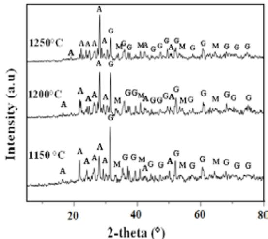
Fig. 1. XRD spectra of samples sintered at different temperatures for 1 h. A: Anorthite; G: Gehlinite; M: Mullite
