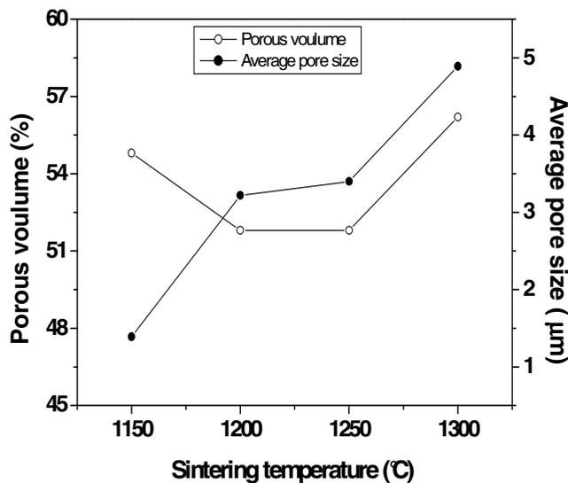
Fig. 2. Porous volume (%) and average pore size vs. sintering temperature.
