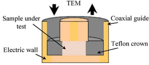
Fig. 2. SuperPol measuring cell.
