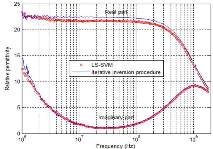
Fig. 7. Permittivity evolution of the ethanol obtained by LS-SVM and iterative inversion method.
