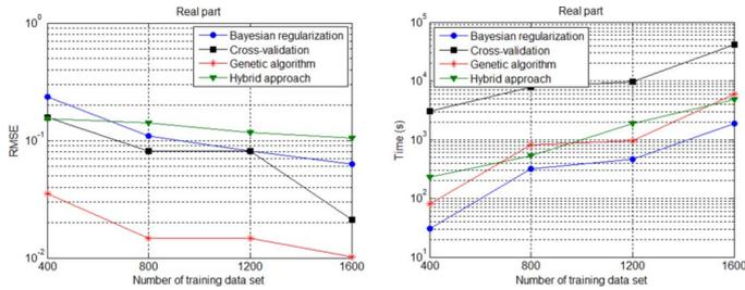
Fig. 5. Error and CPU time on the test set versus the number of training set data (evaluation of  $\varepsilon'$ ).
