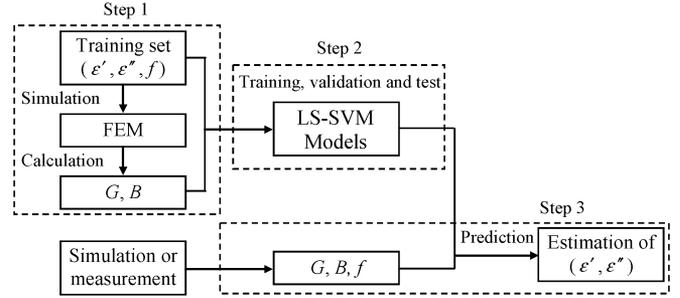
Fig. 4. Microwave properties parameter extracting procedure.
