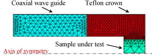
Fig. 3. View of the meshed measurement cell.
